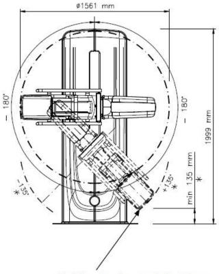
(\*) When the distance of the C-Arm lower edge from the floor is ≤135 mm the rotation range is limited at +/-135° to avoid crushing of the patient feet
