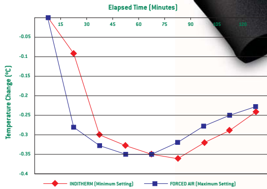
▲ Graph illustrating the comparison between Inditherm Mattress at minimum heat setting, and forced-air patient warming device operating at its maximum heat setting.
