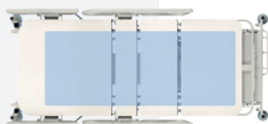
PL-18.3 tunnel for X-ray cassette under the back rest segment PL-18.4 tunnel for X-ray cassette under the bed segments
