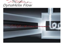
The DynaHelix Flow technology perfectly aligns WBC, RBC and PLT cells for high impedance counting precision using advanced hydrodynamic-focused sheath flow before passing through the aperture. In addition, the DynaHelix Flow totally prevent risk of coincidence or count of blood cell re-entry into the aperture using unique DynaHelix Flow stream. This newly-developed advanced DynaHelix Flow technology greatly improve counting precision and accuracy.
